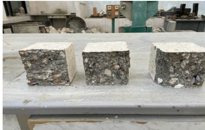
Figure(1): the attack of salts on the bitumen
