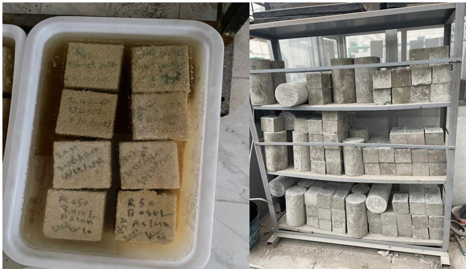
Figure(6): samples of bitumen before immersion with acids and after immersion
