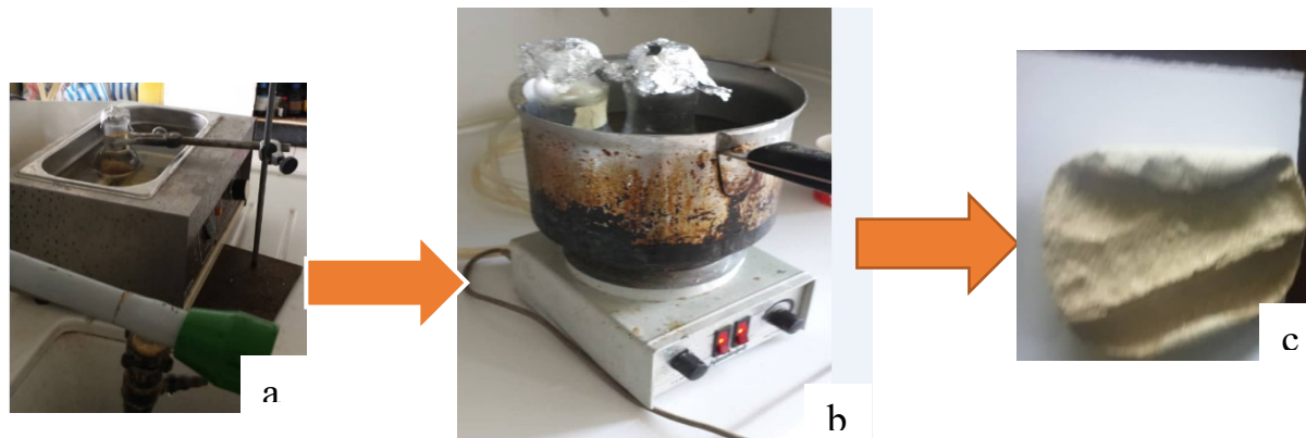
FIGURE 6 Holocellulose extraction (a) Residue 4 (b) Cooking pot in the Magnetic agitaor (c) Holocellulose (Residue 5)
