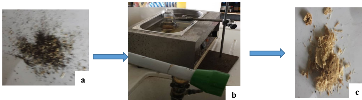
FIGURE 5 Lignin extraction (a) Residue 3 (b) Flax of 250ml and its set (c) Lignin (Residue 4)
