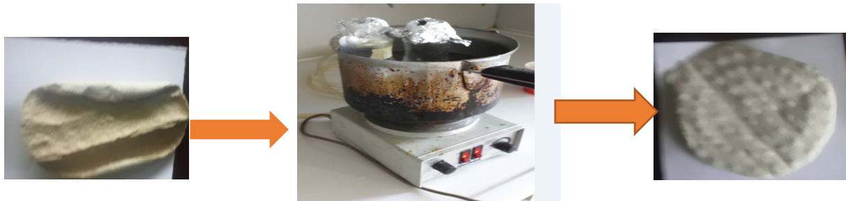
FIGURE 7 Cellulose Extraction (a) Residue 5 (b) Cooking pot in the Magnetic agitator (c) cellulose (Residue 6)
