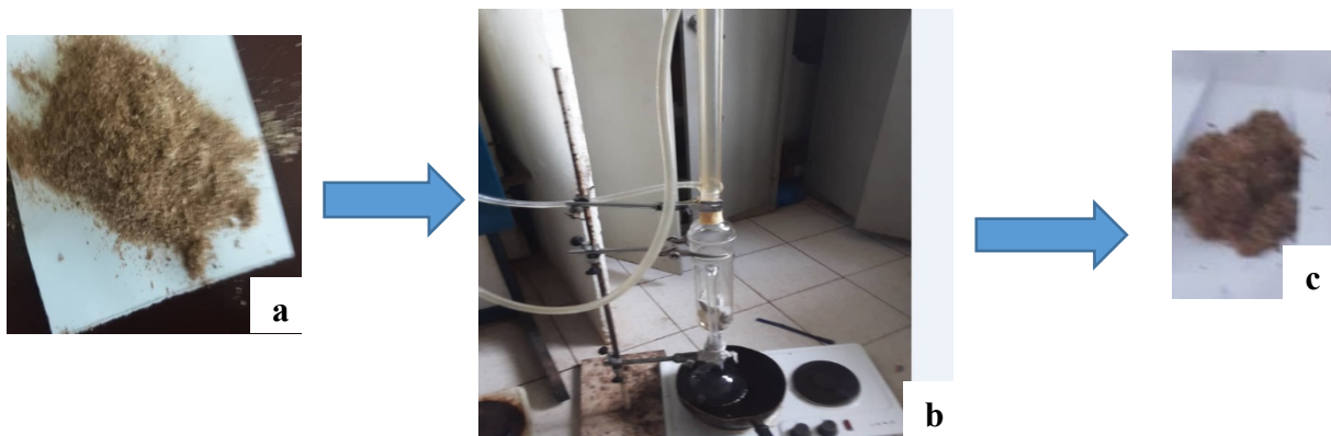
FIGURE 2 Ethanol-Benzene Extraction (a) Dried Powdered of Banana fiber (b) Soxhlet (c) Residue 1
