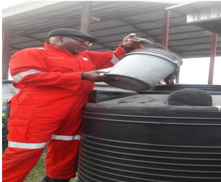
Plate 4: Introduction of Slurry into the Biodigester
