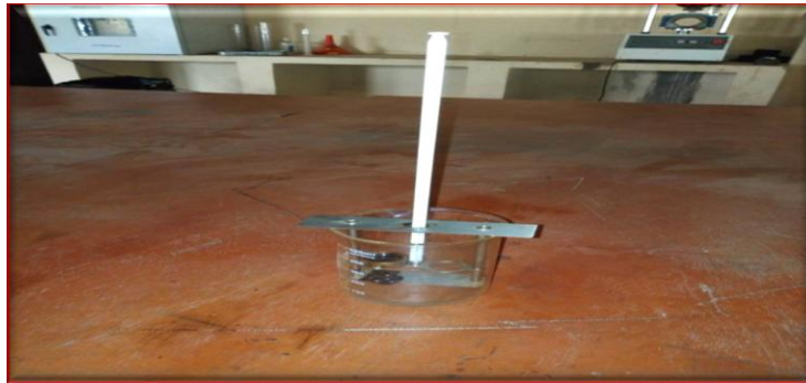
Plate VIII: Ball and ring apparatus used for the test
