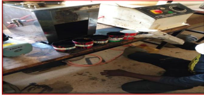
Plate IV: Mixing containers with modified bitumen samples in smaller containers
