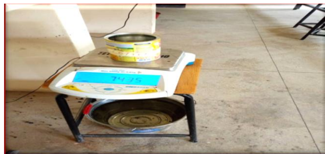
Plate VII: Weighing process for determining relative density using a digital weighing machine
