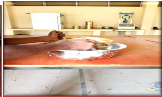
Plate II: Process of sieving of ground bamboo into requisite powder particle size
