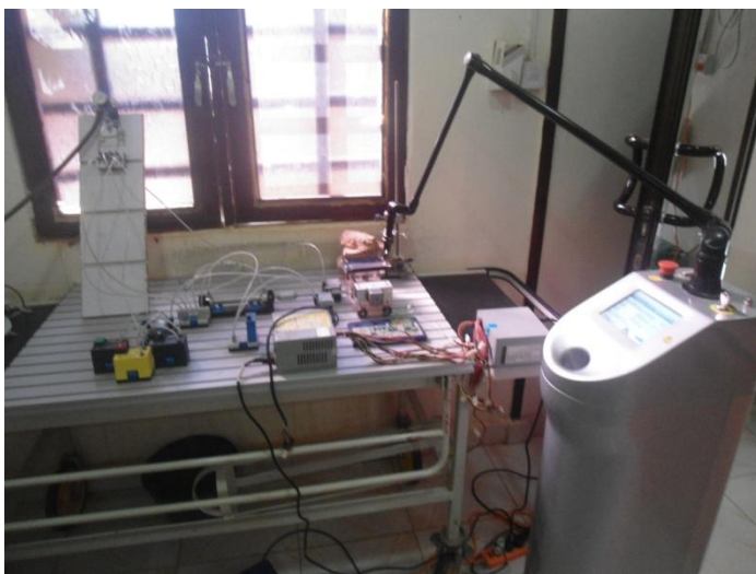
Figure 3: The experimental setup used for laser micromachining of PMMA
