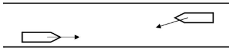
Figure 7: Two ship in avoidance during navigating in confined channel
