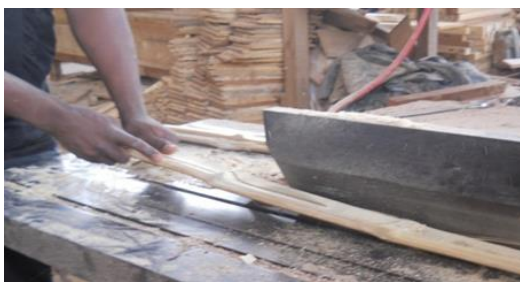
Fig., 4: Splitting of bamboo
