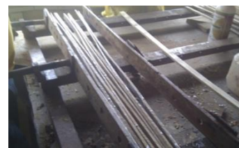
Fig., 9: Gluing and pressing of bamboo strips.
