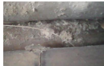
Fig., 1b: group B of bamboo attacked by insect and fungi after the seasoning process for 2months
