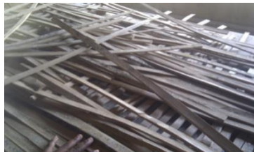
Fig., 8: Drying of preserved bamboo
