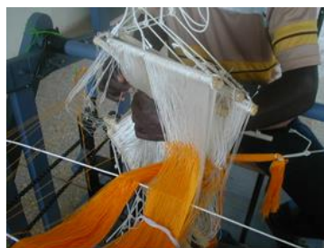
Fig., 12b: Weaver engaged in the heddling process
