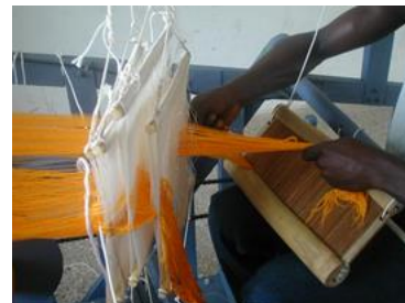
Fig., 12c: Weaver engaged in the reeding process
