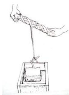
Fig., 11: Beaming by the box method originally used as the warping stone ( Tweso )
