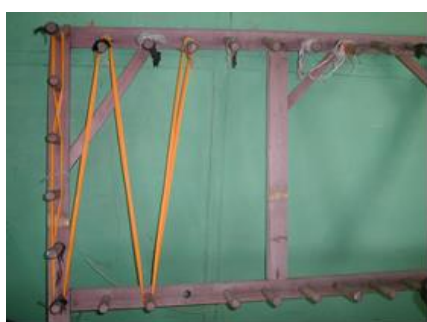
Fig., 10: Warping with the warping board
