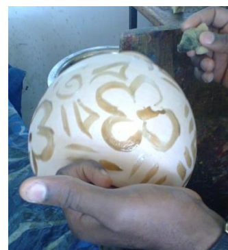
Figure 3: Application of wax on the surface of ceramic ware in form of motives
