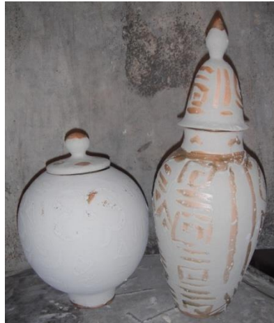
Figure 4: Thick and light applied glaze on waxed biscuit wares at dried stage
