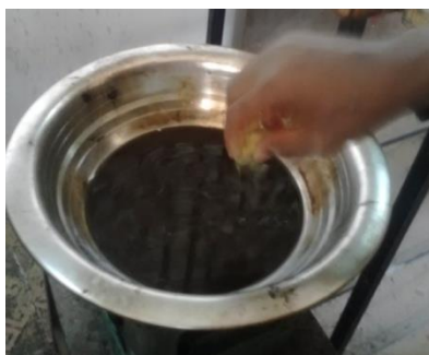
Figure 2: Melted Paraffin wax ready for application
