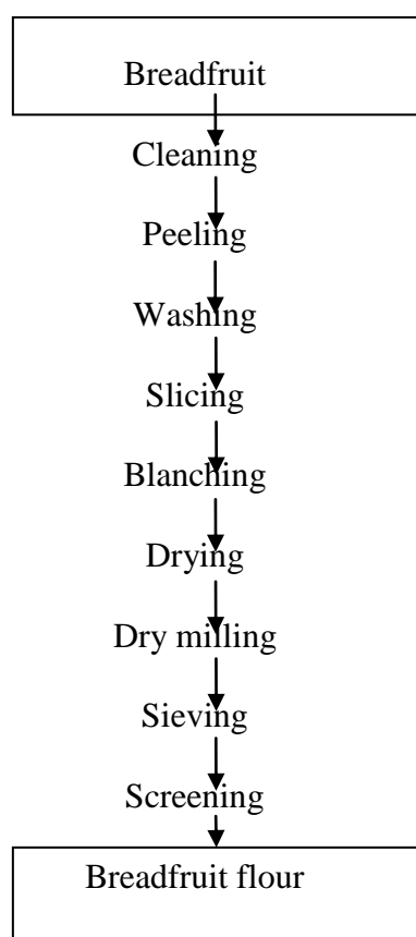
Fig. 1: Flow chart for the production of breadfruit flour.
