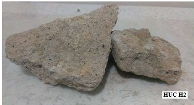
Figure 17. Mortar sample numbered HUC H2 which was taken from Harran City Walls
