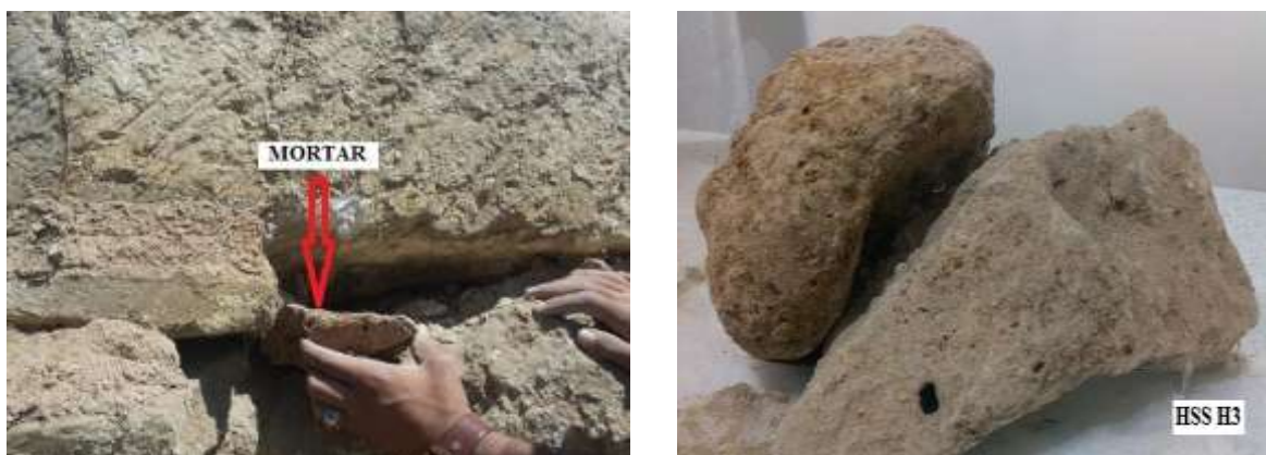
Figure 12. Mortar sample numbered HSS H3 which was taken from Harran City Walls
