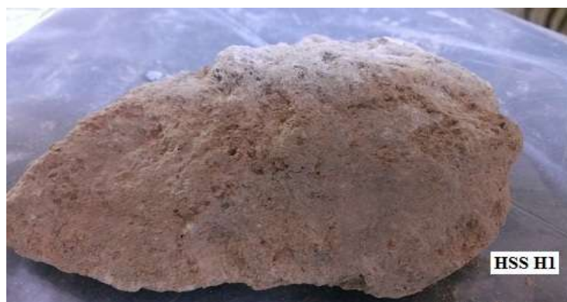
Figure 10. Mortar sample numbered HSS H1 which was taken from Harran City Walls
