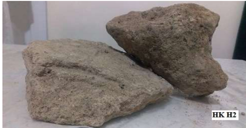
Figure 14. Mortar sample numbered HK H2 which was taken from Harran Castle
