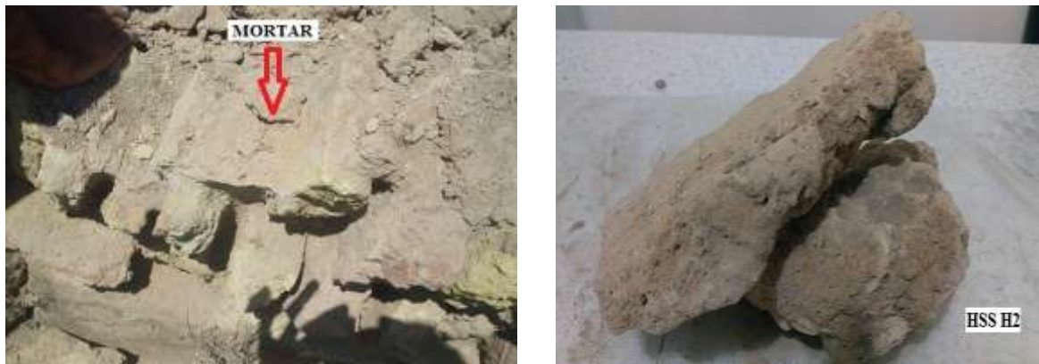
Figure 11. Mortar sample numbered HSS H2 which was taken from Harran City Walls
