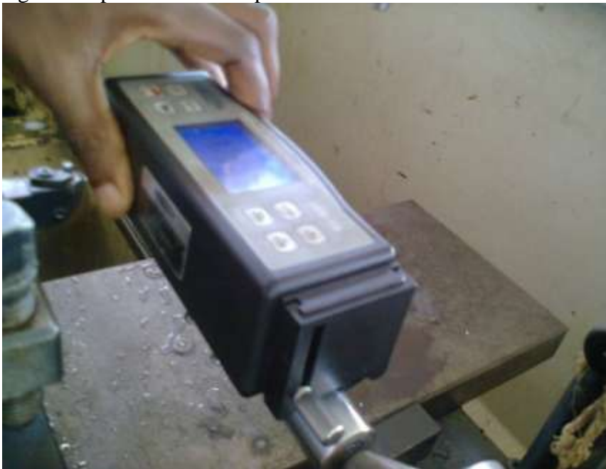
Fig. 3.2 Surface Roughness Tester ISR16
