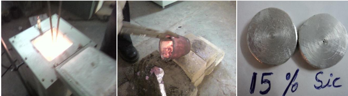
Fig. 1(a) Designed and developed stirring setup Fig.1 (b) Pouring mixture of molten Al and SiC particles Fig.1 (c) Prepared workpieces of Al/SiC-MMCs
