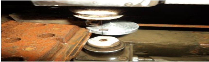
Fig.2 Machining number of Cubes by WEDM
